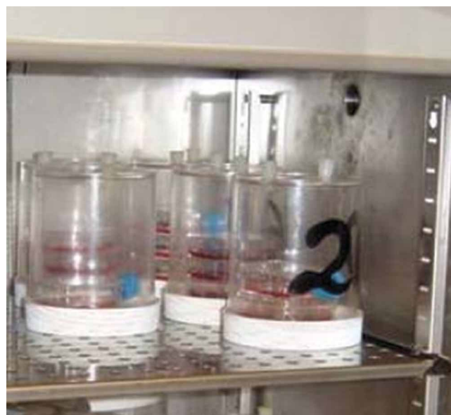
Figure 1 | Low-oxygen chambers in use. Low-oxygen chambers containing flasks and dishes in a normal laboratory incubator can be mixed with dishes cultured in atmospheric oxygen.
