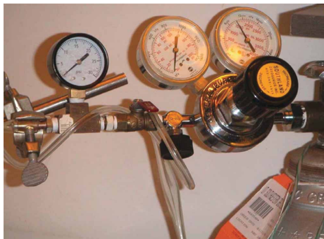
Figure 3 | Low-pressure delivery system. Although a regulator with a second stage capable of delivering 2 p.s.i. can be purchased, one can cobble together a low-pressure gauge with materials available from a local hardware store. We interposed a shutoff valve (with the red handle) so that, once everything is set up, all one needs to do is turn the shutoff valve to on for 2 min to flush the chambers.
