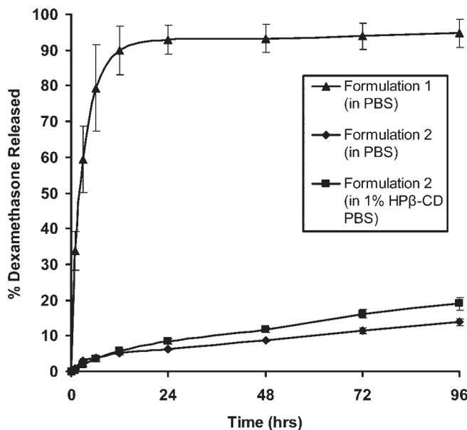
**Figure 1.** *In vitro* release profiles of DEX-loaded millirods of varying formulations. Formulation 1 is composed of 60% PLGA, 16% HP $\beta$ -CD, and 24% DEX complexed with HP $\beta$ -CD (1.7% total DEX). Formulation 2 is composed of 60% PLGA, 38.3% NaCl, and 1.7% uncomplexed DEX. The error bars were calculated from triplicate samples.
