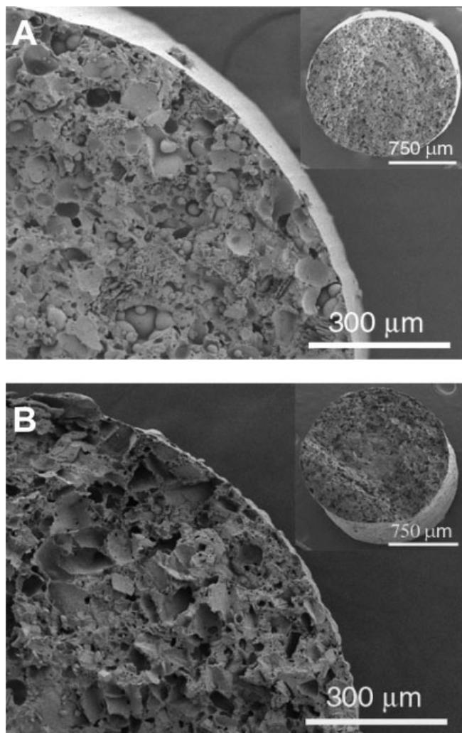
**Figure 2.** SEM analysis of polymer milliroad microstructure after 24-h immersion in PBS buffer. (A) A magnified image of the cross section of a milliroad pertaining to Formulation 1. (B) A cross-sectional magnification of a milliroad from Formulation 2. The insets in (A) and (B) represent low-magnification images of the cross sections of the respective milliroads.
